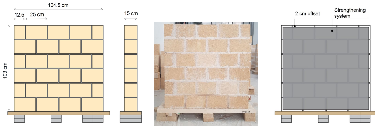
Figure 4. Masonry pattern and strengthening layout.
