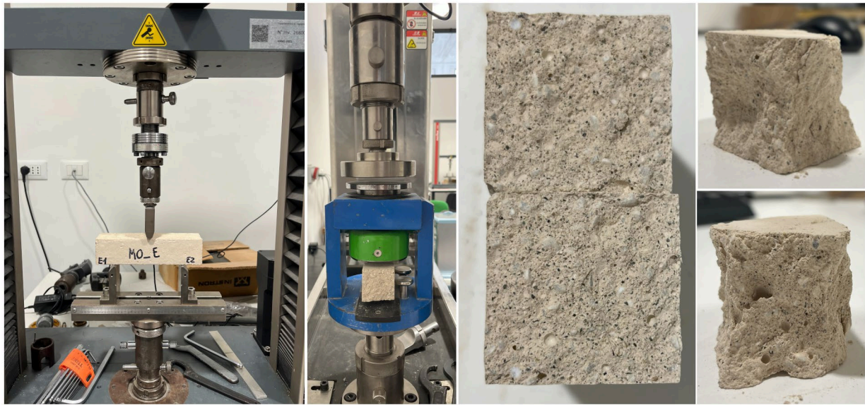
Figure 3. Tests set-up and samples after flexural and compressive tests on mortar pieces.
