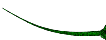
Figure 13 Blade Mode Shape: 1
