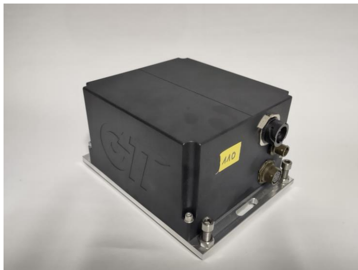
Figure 6. 6C sensor for building health monitoring
