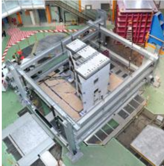
Figure 5. AZALEE shaking table, https://sera-ta.eucentre.it/ta-facilities/ta_f04_cea/
