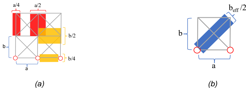
Figure 2. Details of the concrete truss members (a) tributary widths of the horizontal and vertical concrete truss members (b) tributary width of the diagonal concrete truss members
