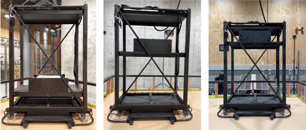
Figure 9 Adjustable centre of mass by changing middle shelf position, "L," "M," and "H" from left to right
