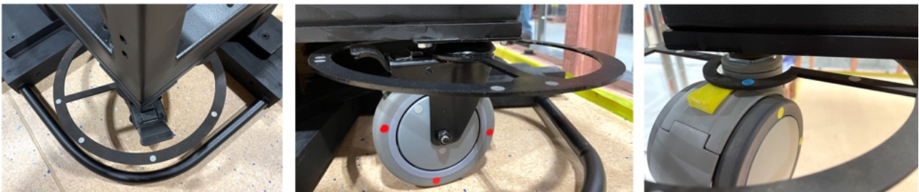
Figure 5 Reflective markers on a disk fixed to caster's fork (left), and disk mounted to the plate-type caster (middle) or stem-type caster (right)
