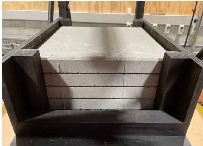
Figure 8 Added concrete blocks to change the specimen's self weight
