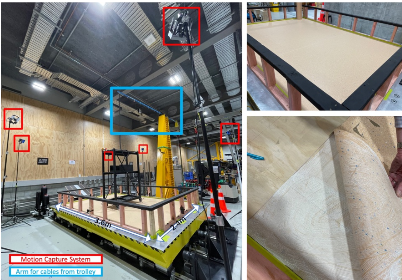
Figure 2 Testing specimen, vinyl flooring and MoCap cameras locations
