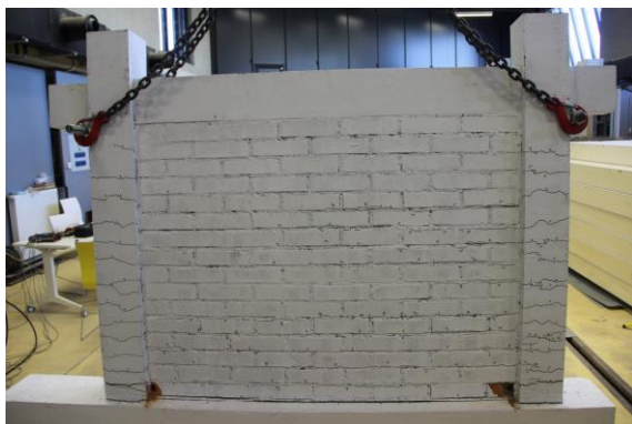
Figure 11. Damage state at final stage of OoP bending tests on test RC frame with masonry infill walls presented photograph (left) by Von Mises strains recorded by ARAMIS (right): a) clay block, and b) clay brick masonry infill wall with tie anchors
