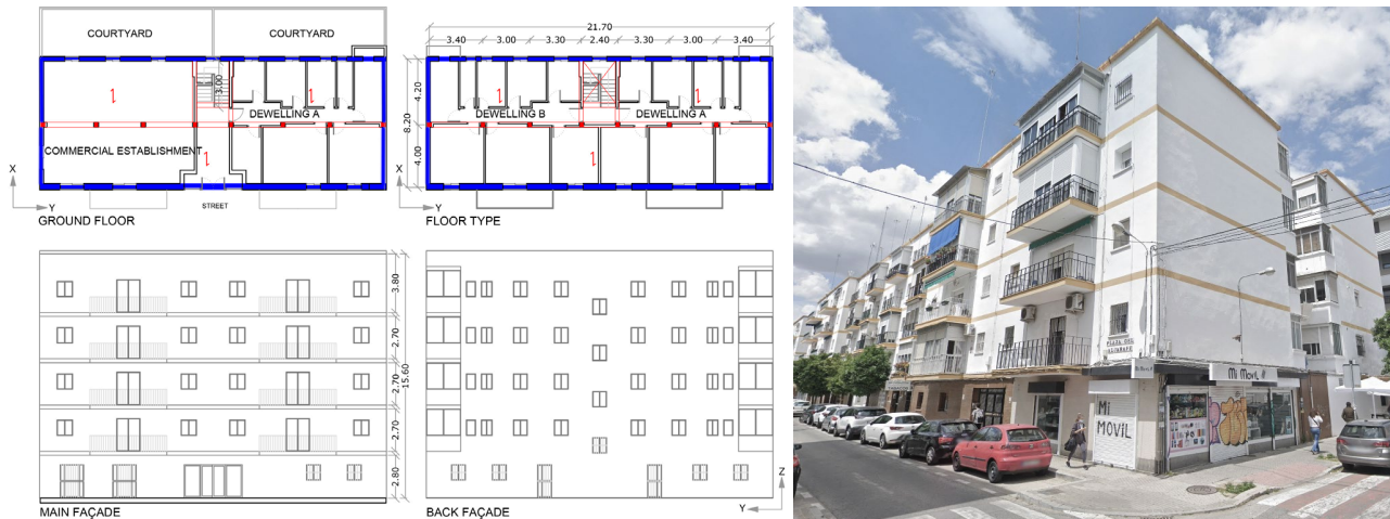
Figure 1. Structural configuration, pointing out in red the interior RC frame and beams and in blue the masonry walls. Distribution in elevation and in plan. Plans and photo of the building by the authors.
