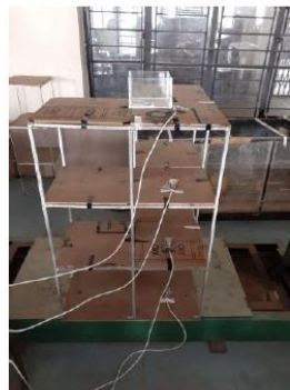
Figure 4: Tank positioned near centre
