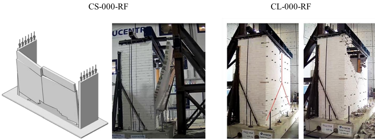
Figure 1: Failure mechanisms of walls CS-000-RF and CL-000-RF observed experimentally.
