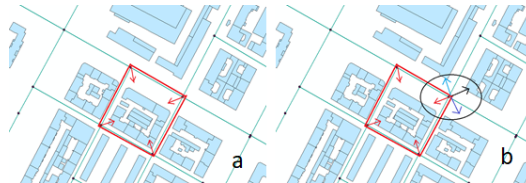
Fig. 3. (a) Water demand Q_{demand,j,w} within a mesh element w in district j , (b) Water demand at node i .
